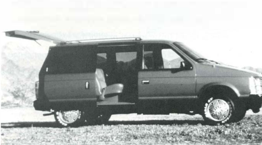
Figure 1 The Chrysler TEVan. Initial production of this electric minivan, the first designed for light cargo or passenger vehicle use, is planned for 1991.
