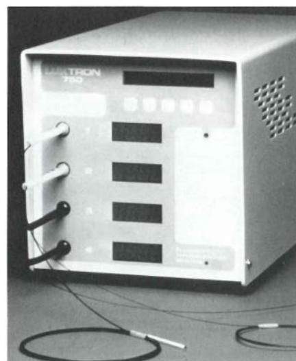
Figure 1 A new device that directly measures transformer winding-conductor temperature, the Fluoroptic thermometer uses a phosphor-tipped probe (foreground).
