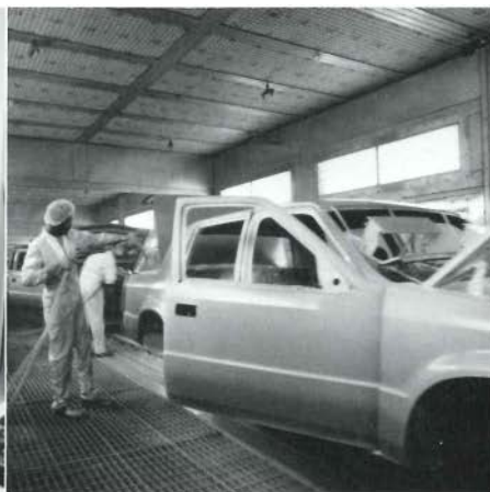
Painters spray interiors, under hoods, in wheel wells; then foil-clad robotic equipment takes over—30,000-rpm rotary spray "bells" and reciprocating spray guns that apply a film of finely atomized paint up to a thickness of 1.8 mils.
