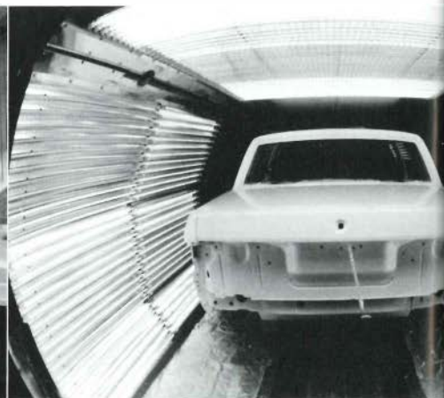
The electric IR oven, located right in the spray booth itself, is the centerpiece of Chrysler's new paint shop. Radiant heat works from the inside out, driving off volatile paint solvents in less than 30 seconds and making a firm base for the 2.4-mil clearcoat that comes next.
