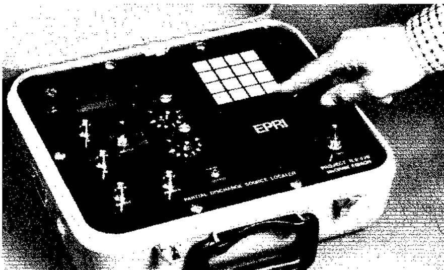
Figure 2 A new partial-discharge detector for transformers is expected to be commercially available from Hartford Steam Boiler Technologies in late 1989.
