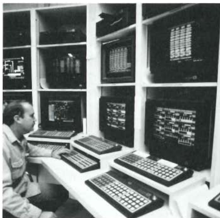
The computer operator keys in the basecoat color and car body codes, thereby controlling the paint spray equipment and programming the timing and intensity of electric IR drying cycles.
