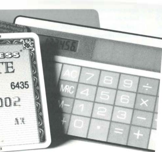
Credit card calculator powered by lithium-polymer laminate battery
