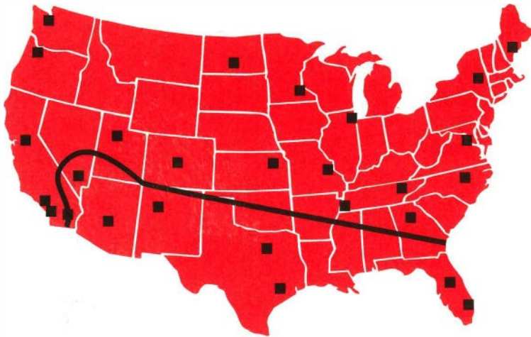
Figure 2 Modeling results for 27 cities were used to project where radiant barriers can be cost-effectively applied. South of the black line, clean horizontal RBs costing 15¢ a square foot are cost-effective in houses that have ceiling insulation rated R-19 or less. (North of the line, such RBs are cost-effective in houses with insulation rated R-11 or less, but higher-rated insulation is typically used in colder climates.) Given higher RB costs, insulation levels above R-19, or a truss rather than a horizontal configuration, the area of cost-effective application shrinks to a smaller southern band.
