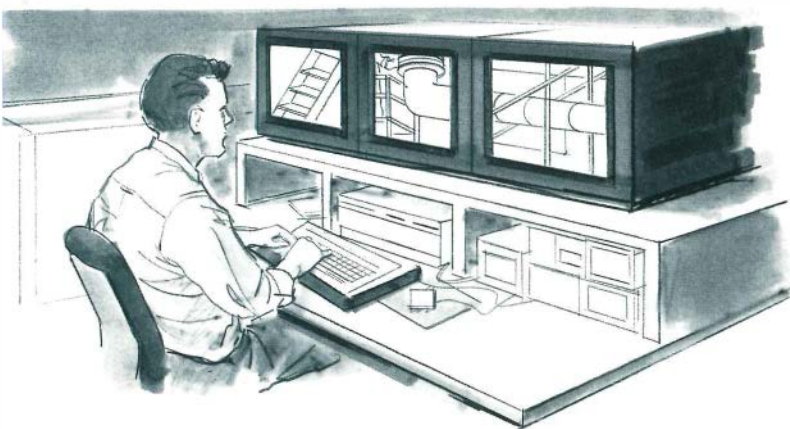
MULTIPLE CAMERAS FOR MULTIPLE VIEWS Nuclear plant video systems combine expensive cameras with a remote control and monitoring console to provide temporary permanent surveillance of work areas or activities. Such systems have substantially reduced personnel radiation exposure during maintenance and inspection tasks at dozens of plants. Shown here is a typical nuclear plant video application involving multiple cameras in a radiation control area.
