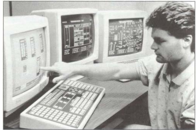
Figure 1 Conventional, mainframe-based simulators (left) for training fossil plant operators are expensive and inflexible. EPRI's new compact simulator technology (right) uses personal computers to provide effective training at much lower cost.
