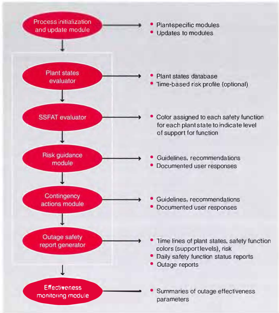
Figure 1 ORAM-TIP software modules and their output. The software divides an outage into manageable stages, or plant states; determines the level of support afforded to seven key safety functions during each plant state; provides risk management and contingency guidelines for each function for each state; and generates easy-to-understand time lines and reports. The user can enter at the appropriate module for planning, tracking, modifying, or reviewing an outage.
