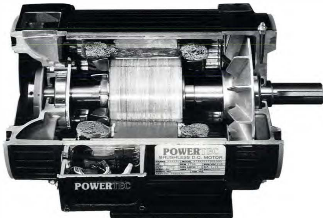
A PEEK INSIDE One advanced motor, now commercially available from Powertec Industrial Corporation of Rock Hill, South Carolina, has ceramic permanent magnets bonded to the rotor shaft. The electronic power converter—a distinguishing feature of all advanced motors—is contained in the small box projecting from the motor casing.
