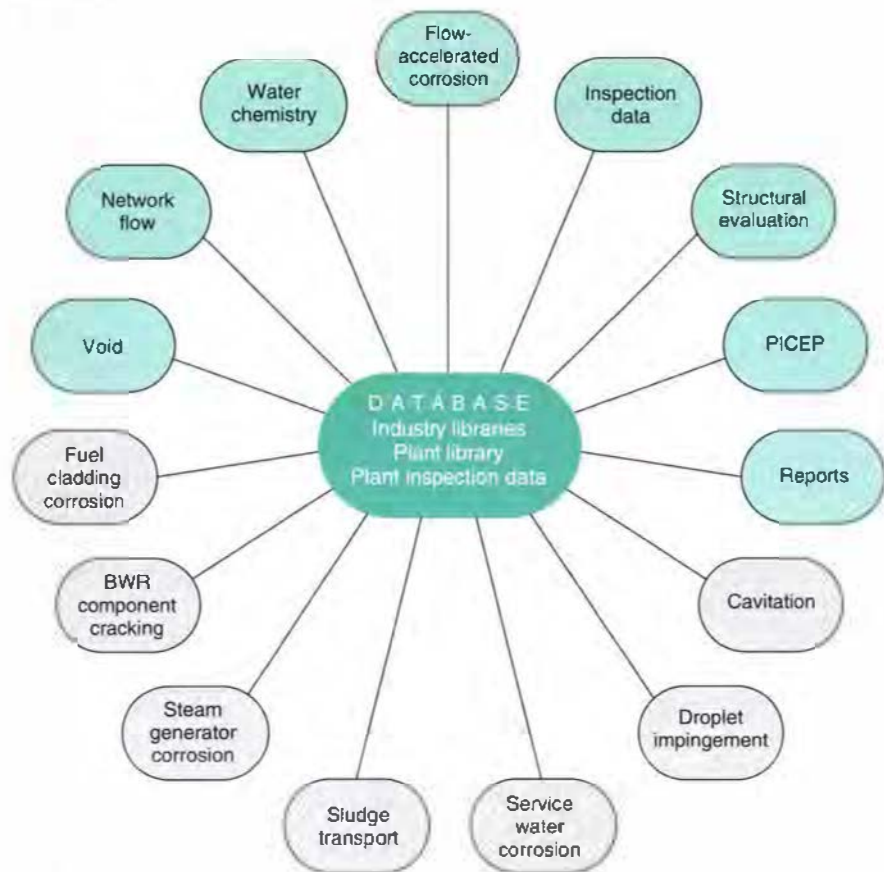
Figure 1 The modular organization of CHECWORKS, in which technology software modules use a common database, is key to its efficient, integrated approach to corrosion control. Version 1.0 (color), scheduled for beta release at the end of the year, will feature seven technology modules focusing on flow-accelerated corrosion, as well as a module for generating reports. Later versions will add the other modules shown.
