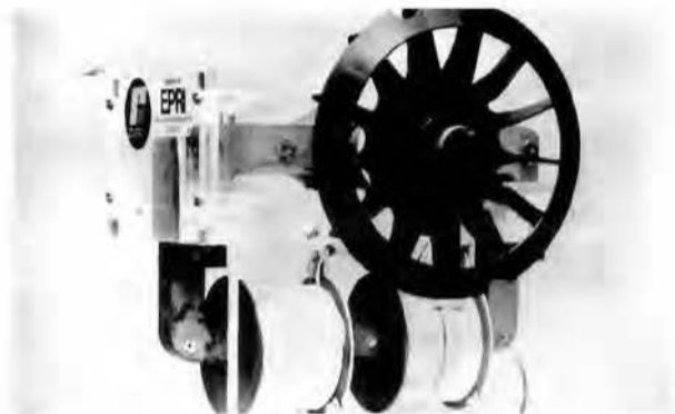
Reliance Electric's HTSC demonstration motor
