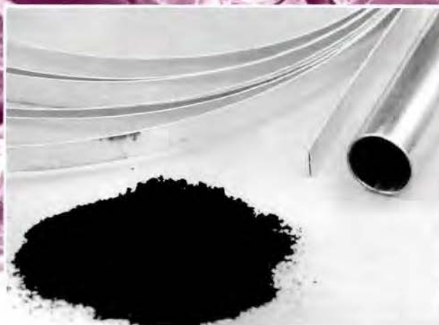
Starting forms for powder-in-tube wire fabrication
