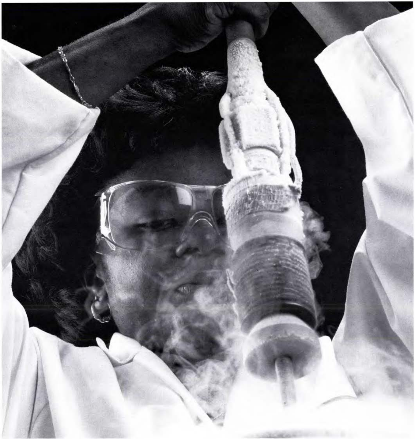
Technician removes HTSC coil from liquid nitrogen bath for testing
