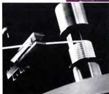
Wire is rolled and wound in pilot manufacturing line
