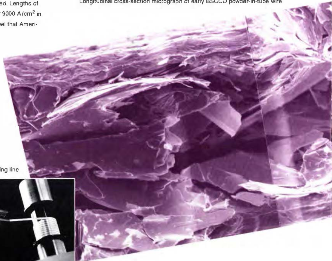
Longitudinal cross-section micrograph of early BSCCO powder-in-tube wire
