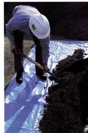
Homer City, Pa. Mike McKelvy "cones and quarters" coal to prepare a uniform sample at EPRI's coal quality evaluation subsidiary, CQ Inc.
