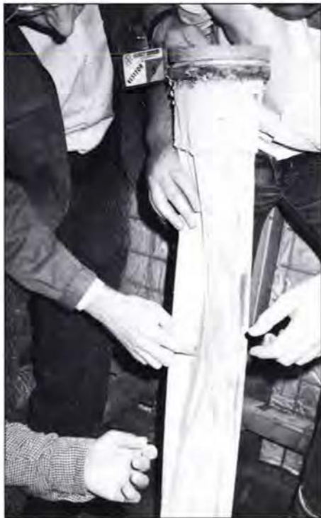
Inspecting particulate dust collected on a COHPAC bag.
