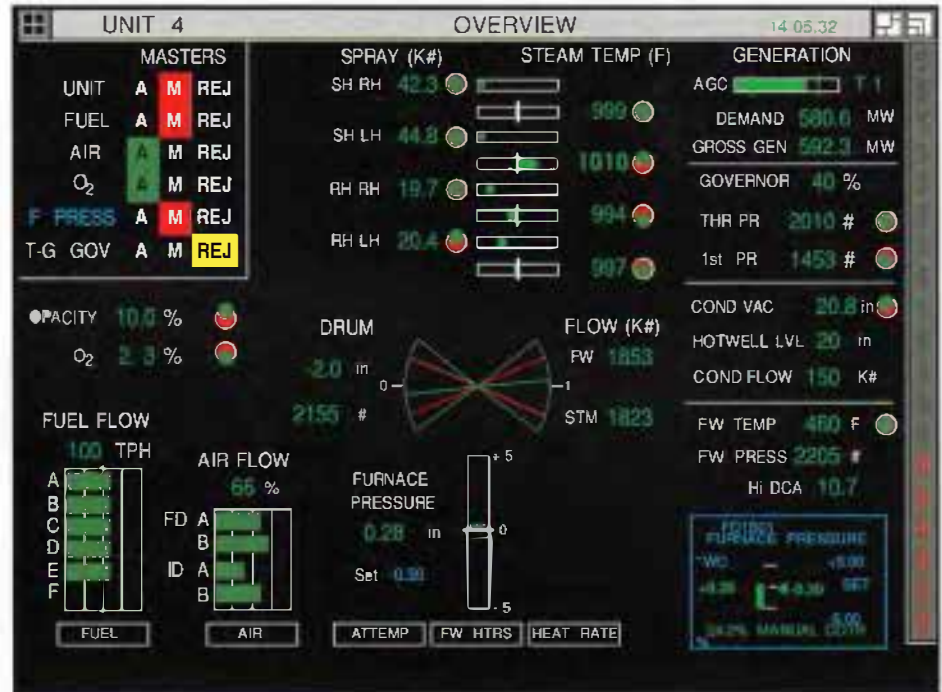
Figure 2 This control system display example gives an overview of plant status. It uses color, graphs, and symbols to provide operators with a broad range of plant information on a single screen.
