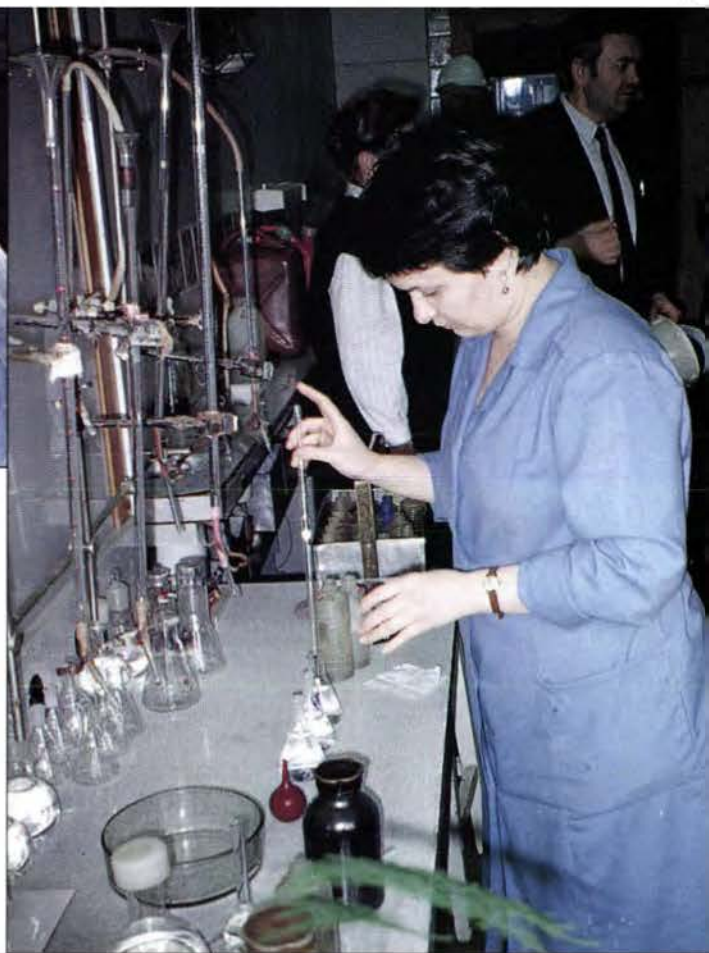
A technician at a Moscow power plant performs a chemical analysis of turbine steam.
