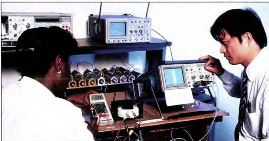
An advanced welding power supply is tested for power quality characteristics.
