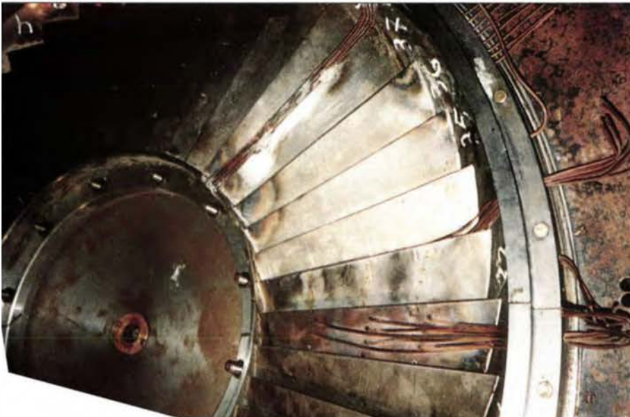
A fully instrumented test turbine at the Moscow Power Institute offers unique opportunities for in-depth analysis.
