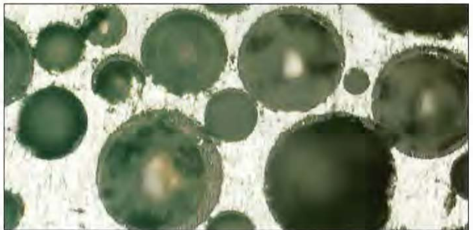
Figure 1 Photomicrographs of aluminum alloy-fly ash (20% by volume) composites: top, \times 550 ; bottom, \times 880 . These show the even distribution of the spherical fly ash particles through the casting volume and the good interfacial contact achieved between the particles and the matrix.
