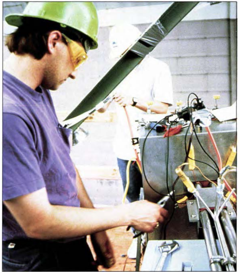
Gas sampling from the inlet and outlet ducts of an electrostatic precipitator
