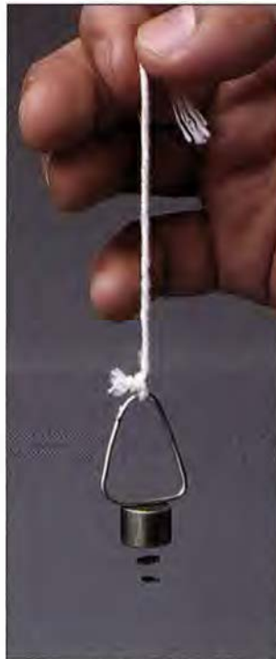
Trapped fields allow two small superconductors to float stably beneath a conventional magnet.
