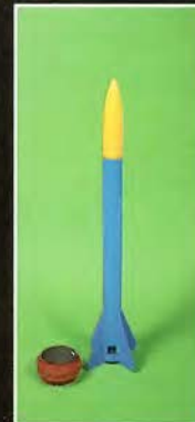
Rocket used to trigger lightning.
