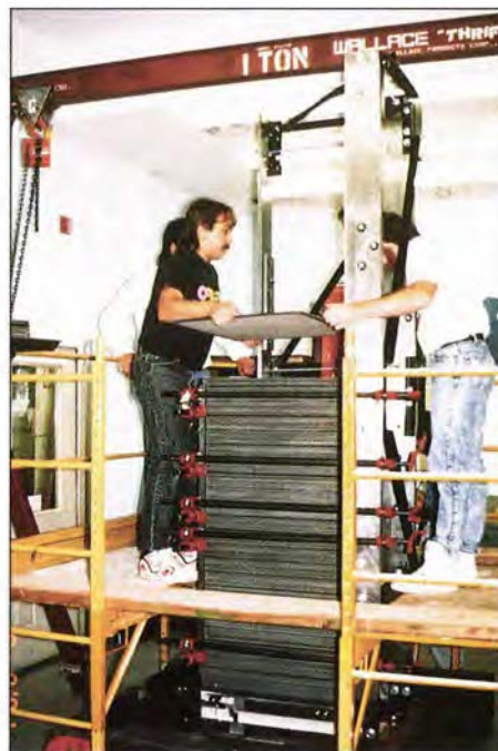
Figure 1 These workers are assembling an external-manifold fuel cell stack designed by Energy Research Corporation. Full-length manifolds for distributing the reactants to the cells and collecting the reaction products will later be fixed to each face of the stack.
