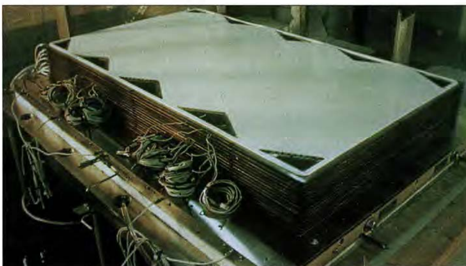
Figure 2 In this internal-manifold stack configuration designed by M-C Power Corporation, the channels created by the triangular openings along the cell edges serve as manifolds for distributing the reactants and collecting the reaction products.
