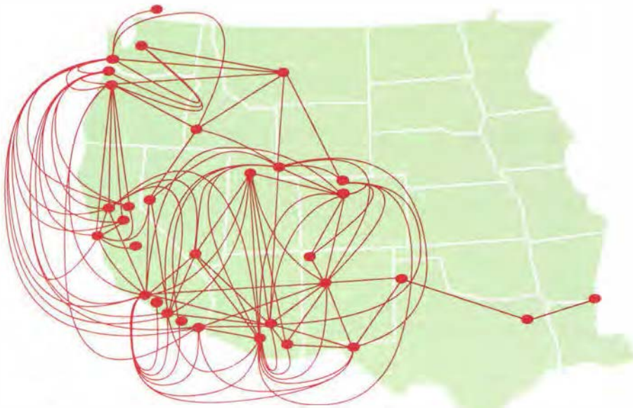
WESTERN SYSTEMS POWER POOL More than 60 utilities are now linked in a wholesale power market that operates through direct interties between about 30 transfer nodes. The power pool facilitates market-based pricing of bulk electricity transactions within limits set by the Federal Energy Regulatory Commission. (Information courtesy of Resource Data International, Inc.)
