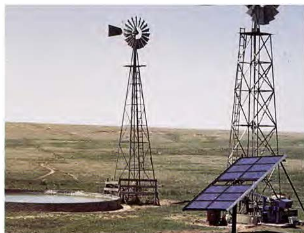
LIVESTOCK WATERING More than 250 PV-powered water-pumping systems have been installed by ranchers, farmers, homeowners, and private organizations in recent years.
