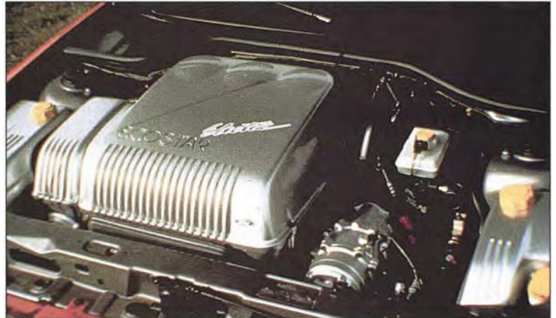
On-board charger (integrated into power electronics box)
