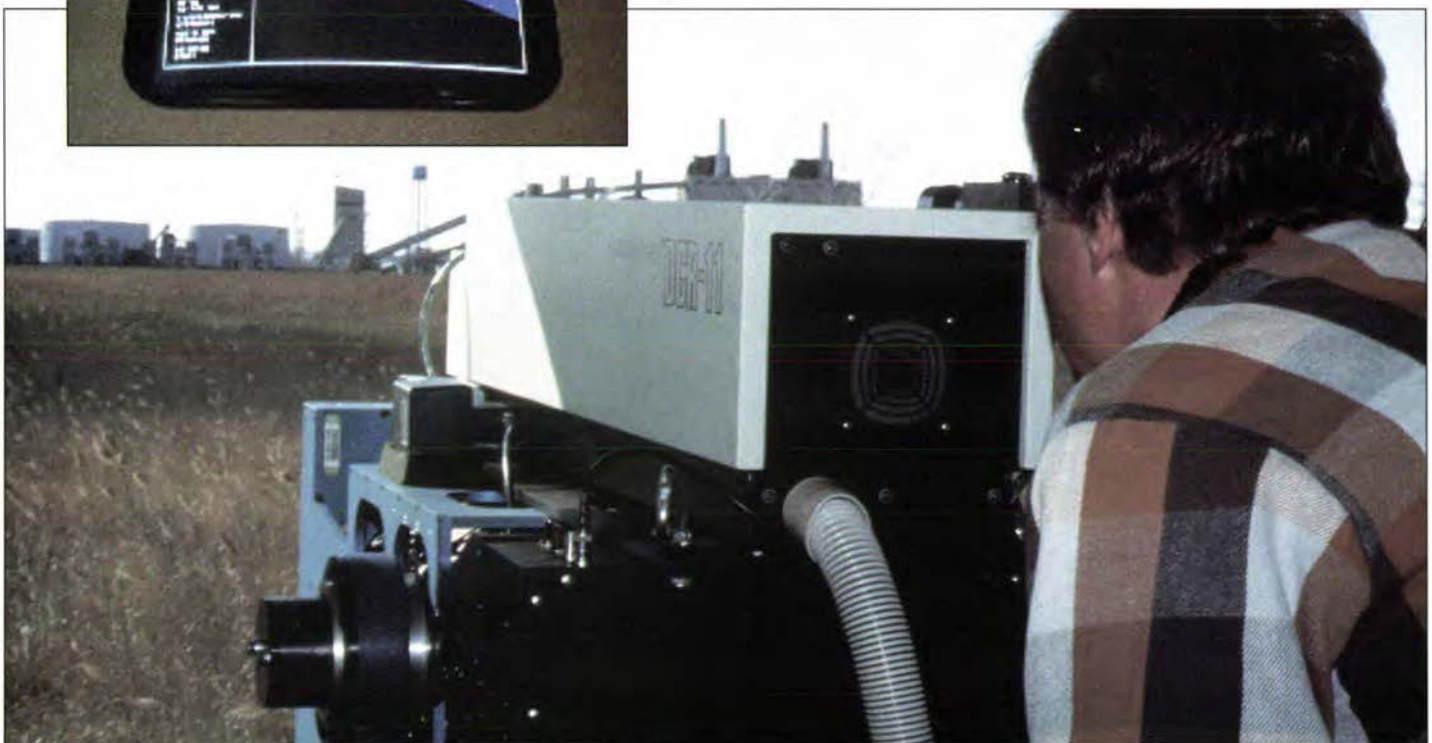
Sighting a LIDAR system to measure plume dispersion at Sayreville Unit 4
