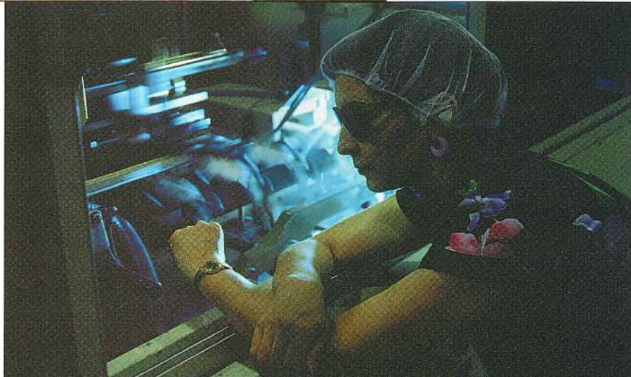
Captive Plastics, Piscataway, installed screen printers with UV curing for the manufacture of pharmaceutical packaging.
