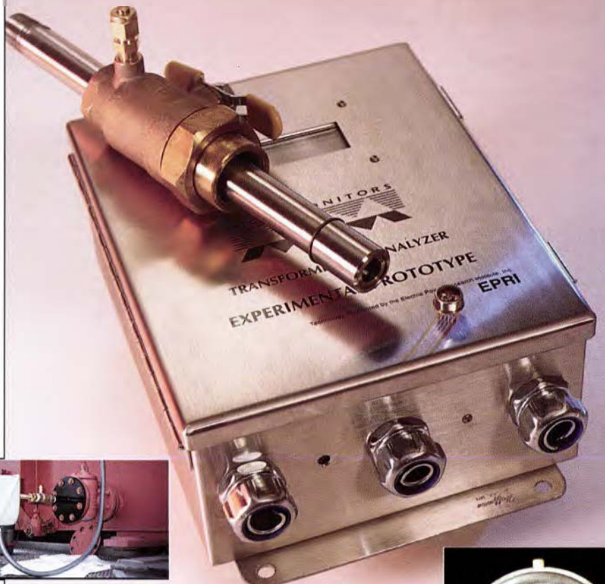
FAULT GAS ANALYZER A new microelectronic device can provide real-time measurement of the four key gases associated with fault currents in transformers. The device features tiny sensors that are inserted directly into transformer oil and transmit data to an externally mounted analysis unit.
