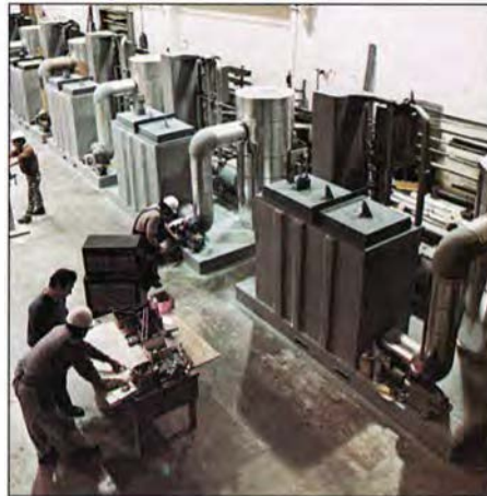
Wahco Environmental Systems, a subsidiary of San Diego Gas & Electric, offers pollution control services and devices, such as these flue gas conditioning systems.
