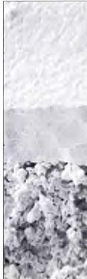
Micrograph of thin-film YSZ electrolyte on porous electrode of solid-oxide fuel cell
