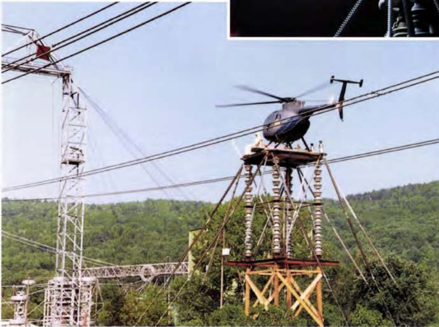
A daytime test shows the entire helicopter setup for a full-scale 800-kV line. Note the bonding spark occurring between the energized conductor and the wire mesh mannequin.
