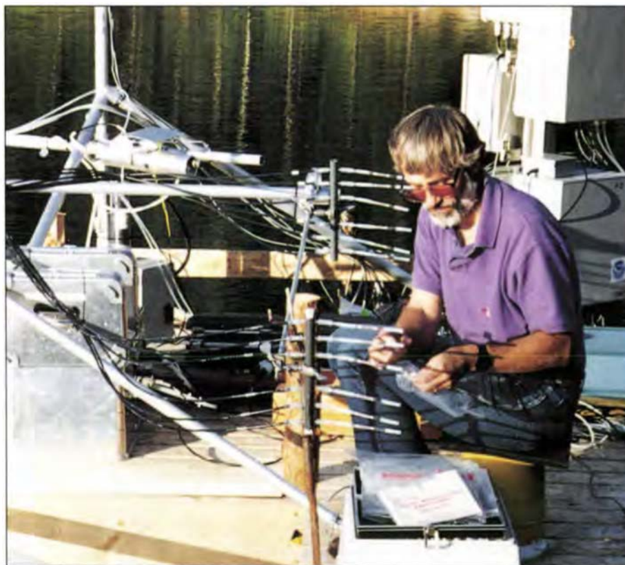
Figure 1 A specialized flux chamber is used to take mercury measurements at an air-lake interface. This new tool is helping improve our understanding of the movement of mercury to and from surfaces. Measurements over soils, grasslands, and lakes are showing that under some conditions the net movement of mercury is from the surface to the atmosphere. Lakes in particular may be very active reemission zones during the summer.
