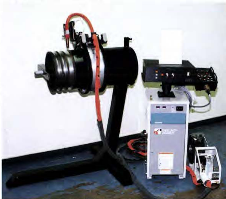
Figure 2 This advanced automated pipe-welding system developed by EPRI and Magnetech combines an orbital tracking mechanism for out-of-position welding and a commercially available power supply with a "fuzzy logic" control feature that greatly improves arc stability.
