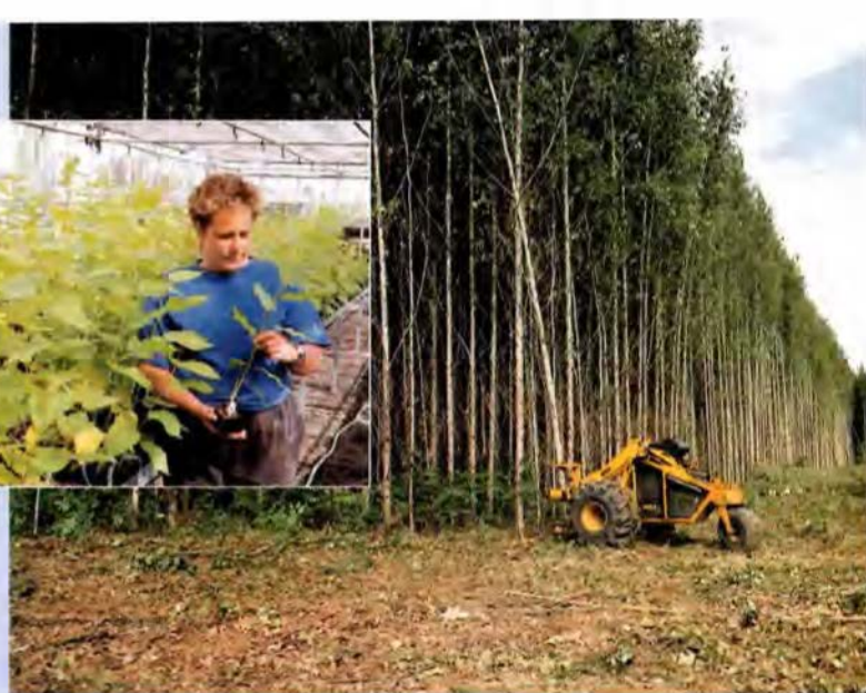
At the Lower Columbia Fiber Farm, a feller-buncher harvesting machine cuts trees and lays them in bunches for later chipping.
