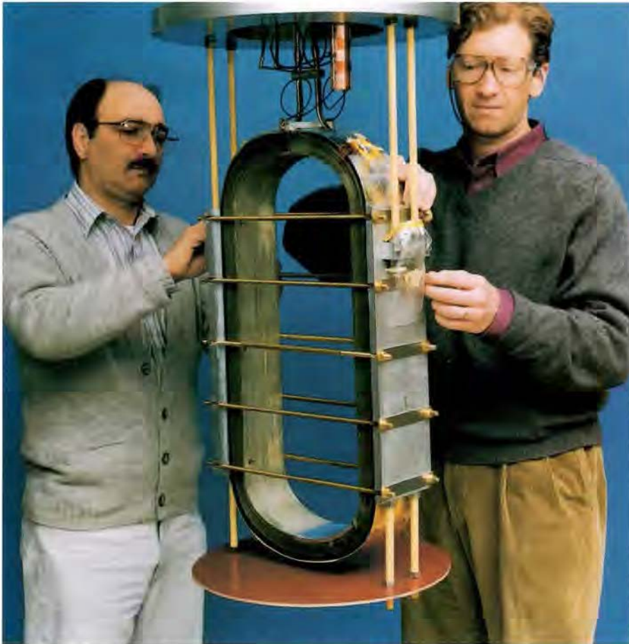
SUPERCONDUCTING RACETRACK FOR AN HTS GENERATOR A team of specialists at General Electric's R&D Center in Schenectady, New York, designed, built, and successfully tested this prototype HTS generator racetrack coil earlier this year. The coil was made from some 2400 meters of BSCCO tape manufactured by Intermagnetics General Corporation. Suspended in a vacuum and cooled with helium gas, the coil was tested at temperatures ranging from 16 to 77 K. It achieved steady-state currents of 34 A at 25 K and 30 A at 20 K. The coil was produced as part of the first phase of a government-industry program targeting the development of high-efficiency, low-cost HTS generators for electric utilities.
