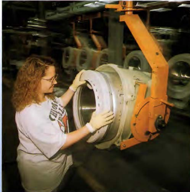
A worker at Maytag's Newton, Iowa, plant assembles the Neptune's inner tub.
