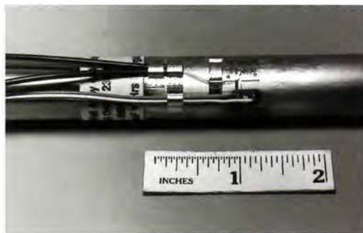
Strain gage installed on tube specimen
