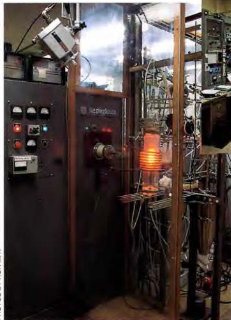
SRI's radio-frequency induction furnace for heating materials samples or wafers to over 2000°C
