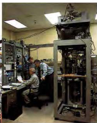
High-temperature mass spectrometer for materials characterization
