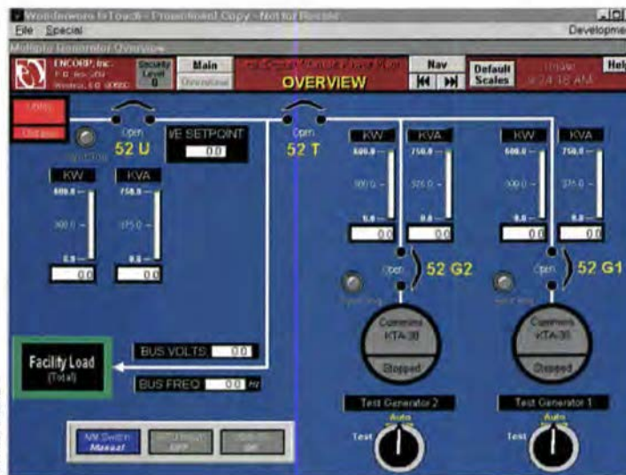
Encorp's Virtual Power Plant software is designed to let users monitor and control multiple remote standby (emergency) generators at various locations via phone lines or other means of communication. PacifiCorp Energy Ventures plans to use the Virtual Power Plant network to dispatch small generators at customer sites as peaking capacity.
