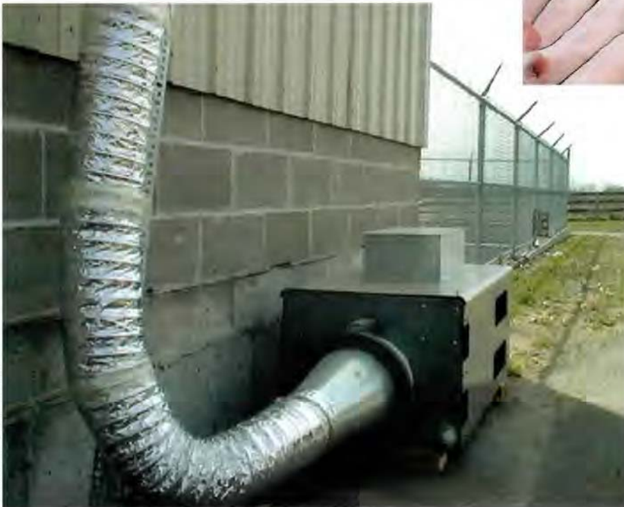
Prototype pulsed-discharge reactor
