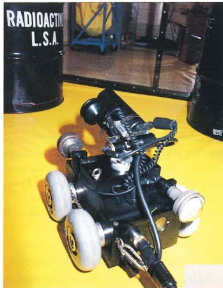
Camera- and sensor-equipped remote inspection robot
