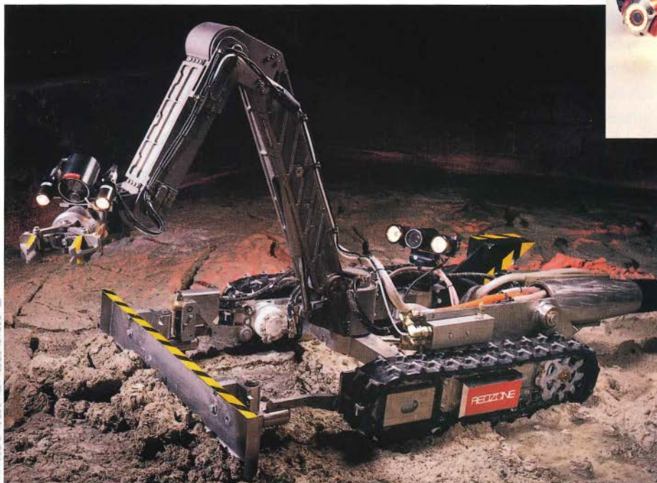
Houdini—a hydraulically powered, bulldozer-like mobile robot for tank-waste retrieval
