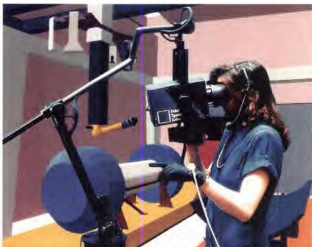
This virtual reality tool can simulate a disaster site in three dimensions for training purposes. EPRI and Sandia National Laboratories are cooperating to identify other advanced Sandia-developed technologies that could be modified for disaster mitigation applications.
