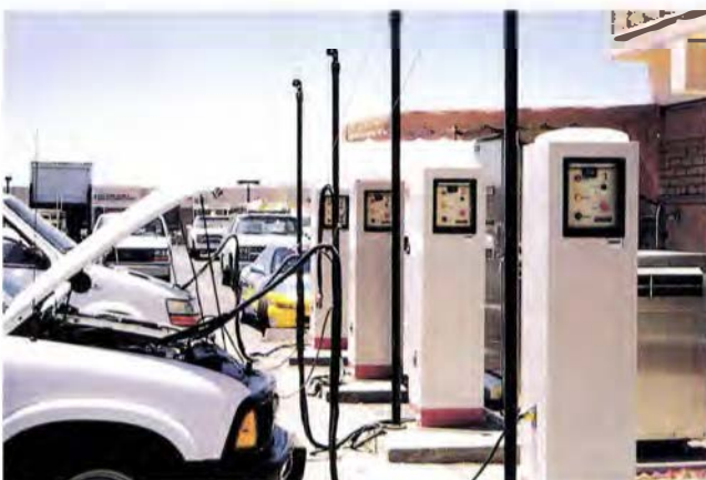
EVs connected to sequencer stations of a Norvik Minit-Charger (behind stations)
