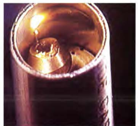
A state-of-the-art laser welding technique can permanently repair cracked steam generator tubes that ordinarily would be sleeved or plugged. This device, being marketed by ABB, employs an EPRI-patented rotating optical coupler—which allows the precise alignment of a laser beam—and a rotating weld head mounted at the end of a fiber-optic cable. Melting an alloy wire, the laser can create a uniform 2–3-inch (5–7.5-cm) weld over a damaged area in about a minute.
