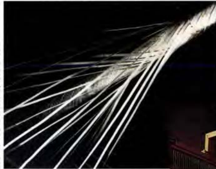
American Superconductor’s HTS tape is fabricated into a stranded conductor assembly by Pirelli Cables and Systems, using modified conventional-cable equipment. The machine on the right then wraps the conductor assembly with thermal insulation made of metallized polyester film.
