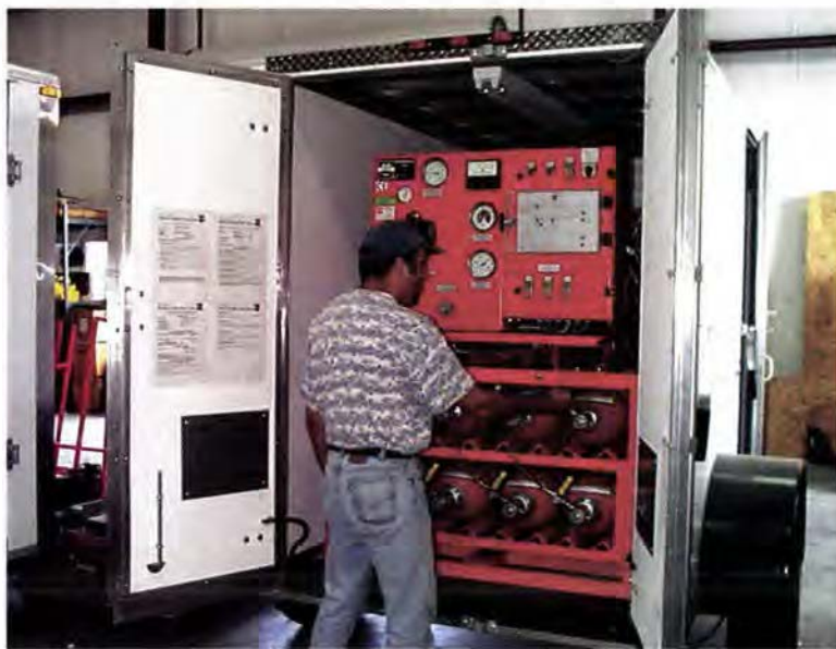
EPRI has helped promote the use of movable SF 6 recycling carts, such as this model, for temporarily containing gas removed from deenergized high-voltage equipment before either inspection by conventional methods or repair.
