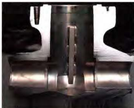
A chromium-plated valve body
