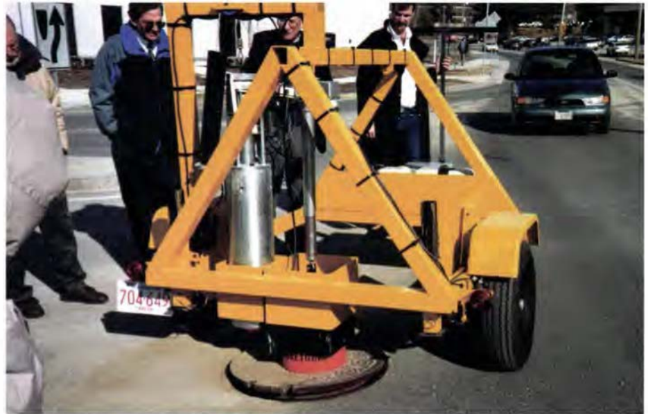
A manhole cover is lifted by the remotely controlled system's electromagnet during trials in Boston. The RAM impact hammer is the vertical cylinder to the left of the magnet.
