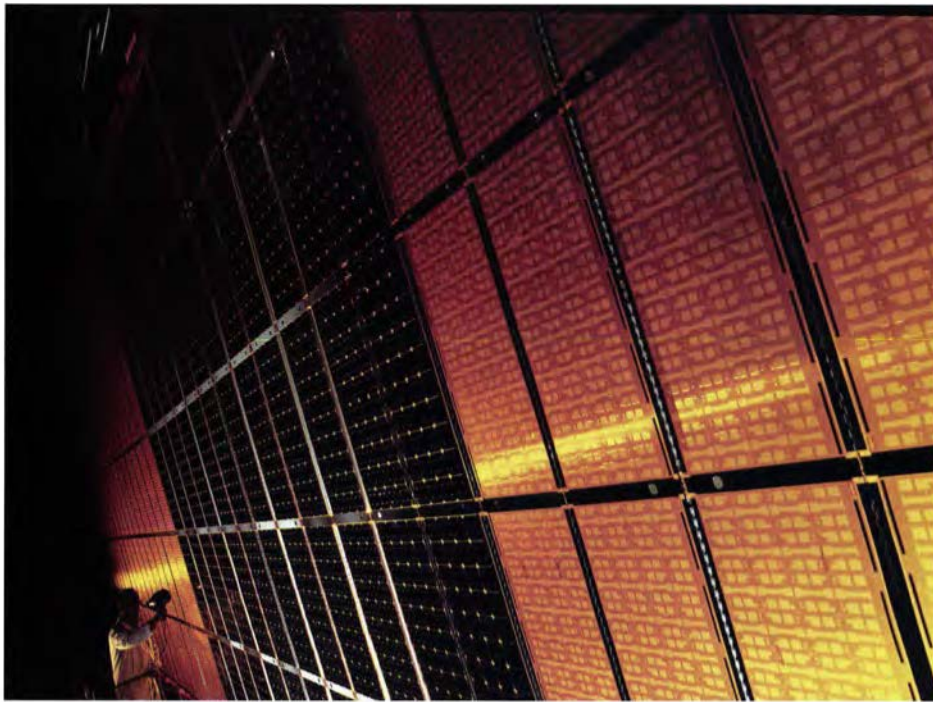
The photovoltaic arrays now used to power satellites may be either rigid structures with crystalline PV modules or flexible thin films that can be unrolled in orbit. Those shown here, designed for the International Space Station by Lockheed Martin, consist of thousands of individual solar cells on a flexible backing. Such current-technology arrays are very expensive and provide limited power. To make large-scale space-to-Earth transmission of solar power commercially attractive would require producing arrays of thousands of square meters at greatly reduced costs—more than an order of magnitude lower than today's.
