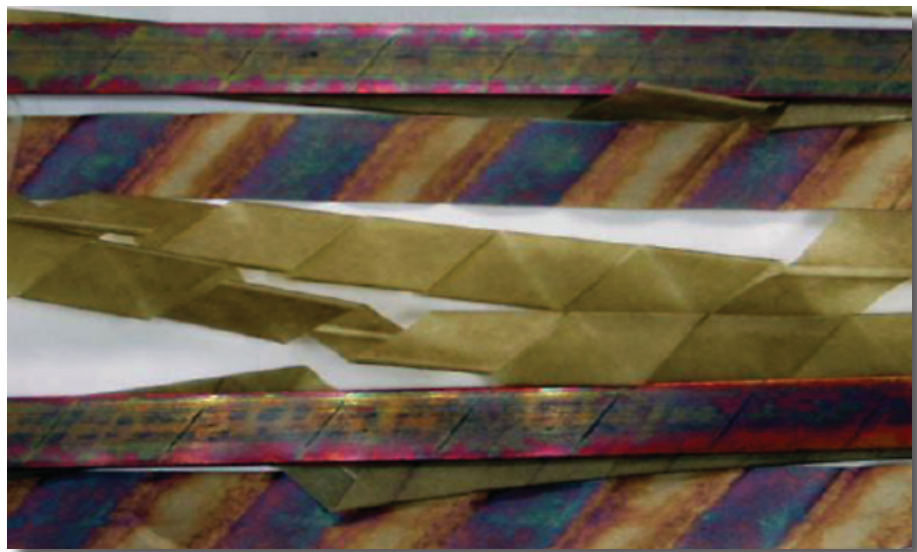
Copper sulfide deposits on insulating paper from a failed transformer.
