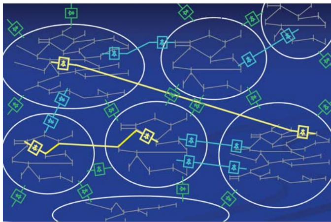
A segmented power grid would be made up of asynchronously operated ac sectors (oval shapes) linked by dc "shock absorbers" (green rectangles) in the form of back-to-back VSC-based dc controllers. Full implementation of the concept may include conversions of existing ac lines to dc (blue lines) and the addition of long-haul HVDC lines (yellow lines).
