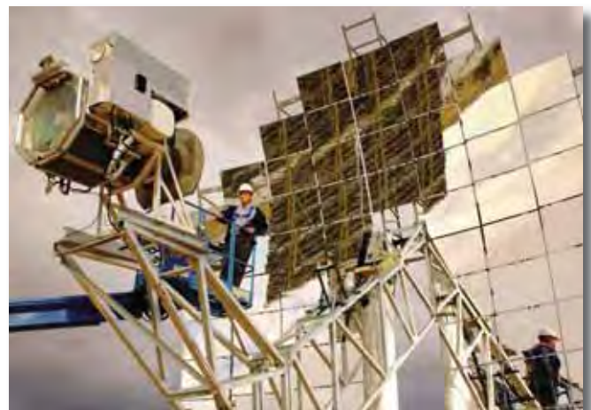
Sandia National Laboratories is evaluating solar dish-Stirling STE systems at its National Solar Thermal Test Facility in Albuquerque. The dish units, which are automated to track the sun, concentrate heat on a Stirling engine, which drives an electric generator. (photo: Randy Montoya)
