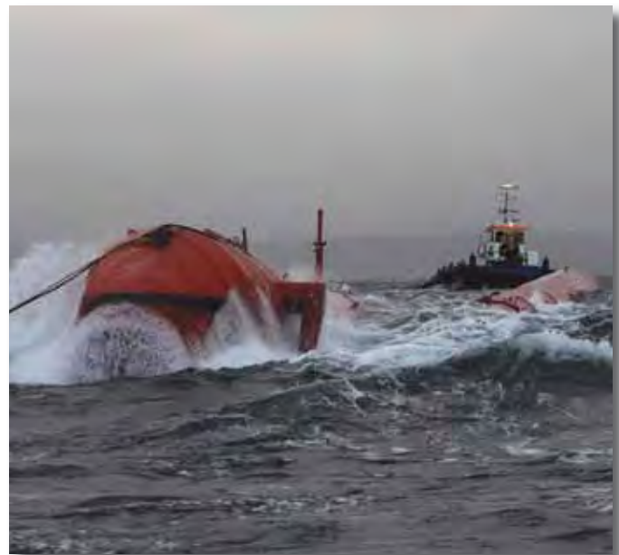
The Pelamis wave energy converter is a string of floating cylinders linked by hinged joints. The wave-induced motion of these joints pumps high-pressure oil through hydraulic motors that drive electric generators to produce power. (photo: Ocean Power Delivery Ltd.)
