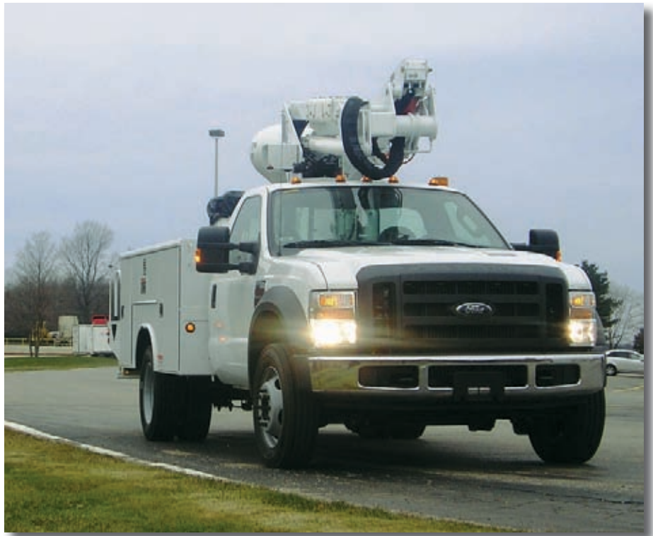
EPRI is leading a broad inter-industry program to develop a PHEV “trouble truck” for servicing utility distribution systems. Based on a Ford F550, the truck will provide 6 to 8 hours of standby work time with minimal engine idling and, in a high-idle mode, will generate up to 5 kW of ac power to provide grid services in the field.
