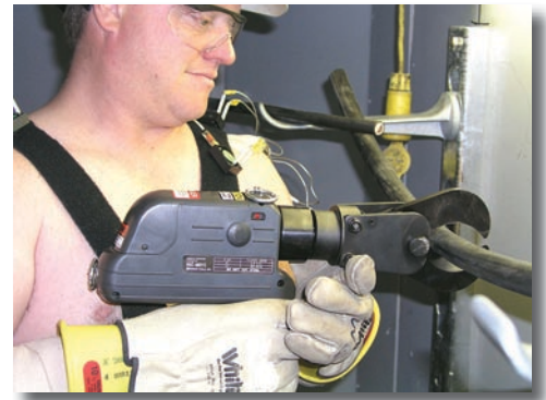
Measurements of muscle activity show that a switch from manual to power tools, such as a battery-operated cable cutter, can significantly reduce strain on the shoulders; prevention of a single chronic shoulder injury could easily pay for the power tool.
