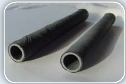
Westinghouse prototype SiC-wound fuel cladding
