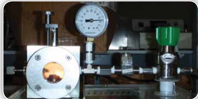
Tests involving high-pressure water jets showed no discernible difference between diamond nanofluids and a water control in the cavitation erosion of test samples.
