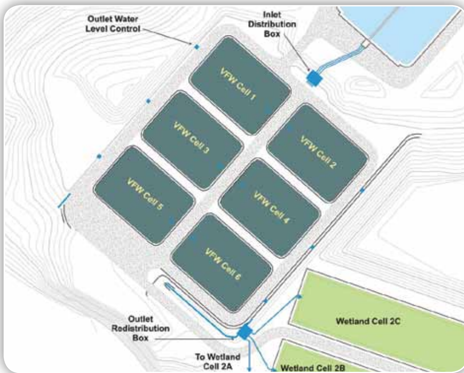
Duke Energy plans to modify an existing FGD wastewater treatment system in North Carolina with six full-scale vertical flow wetland cells.
