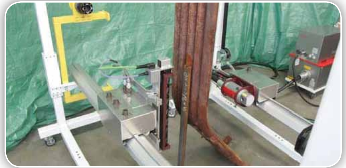
A motion control system keeps the X-ray tube (right) and the digital detector (left) in alignment as they scan boiler tubes for corrosion fatigue cracking.
