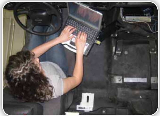
Studies showed that a computer mounted on an articulating arm just to the right of the steering wheel (bottom right) causes the least twisting, stretching, and discomfort.
