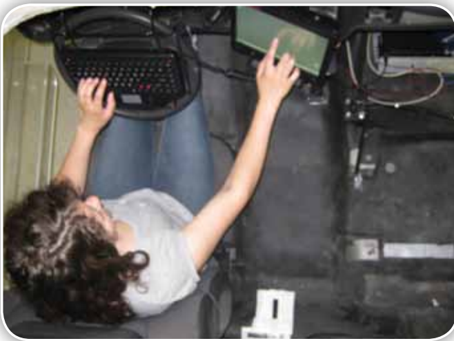
Studies showed that a computer mounted on an articulating arm just to the right of the steering wheel (bottom right) causes the least twisting, stretching, and discomfort.
