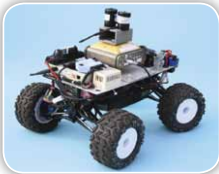
Scotty, a mobile light-measurement robot, performs accurate, timely, and repeatable measurements of LED light levels.
