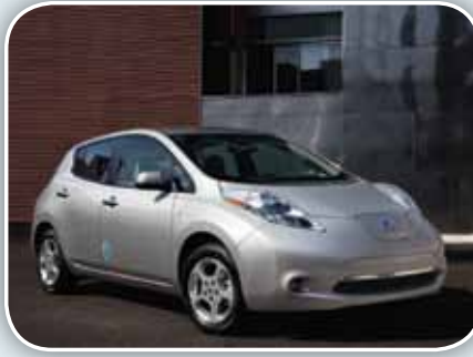
The 2011 Nissan Leaf is a 100% battery electric vehicle with an EPA-rated range of 73 miles. It can use a portable 120-volt charger, but most drivers will likely opt for a dedicated wall-mounted 240-volt charger that can completely recharge the battery from “empty” in less than 8 hours. Photo courtesy of Nissan.
