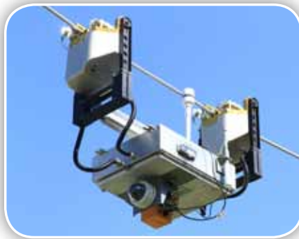
Ti, a transmission line inspection robot, can traverse 60 miles (96.6 km) of line at least twice a year, collecting high-fidelity information that utilities can act on in real time.
