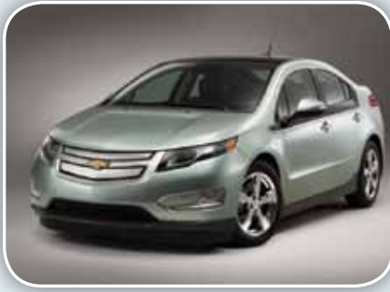
The GM 2011 Chevrolet Volt is a plug-in hybrid. It has an unlimited driving range with its gasoline engine and an EPA-rated range of 35 miles on its battery. It will recharge from “empty” in about 8–10 hours using a 120-volt portable charger or in 3–4 hours from a dedicated 240-volt charger. Photo courtesy of Chevrolet.
