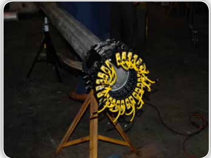
Guided wave sensors installed on piping mockup
