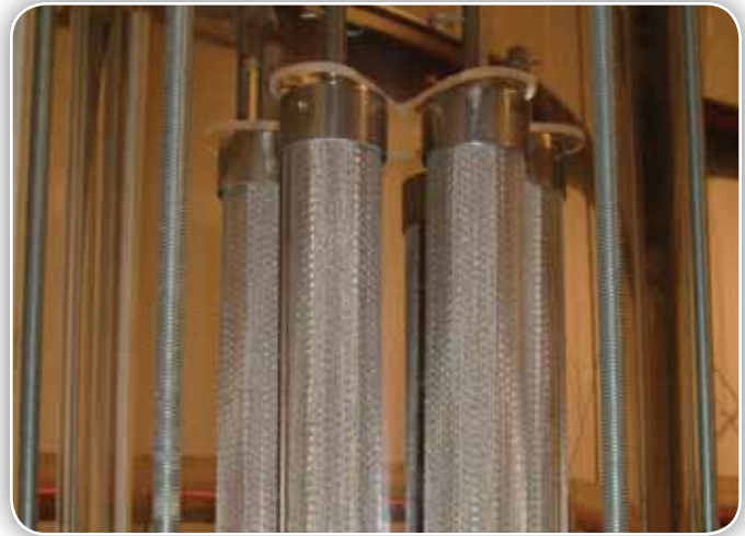
Experimental cobalt sequestration column used in resin testing
