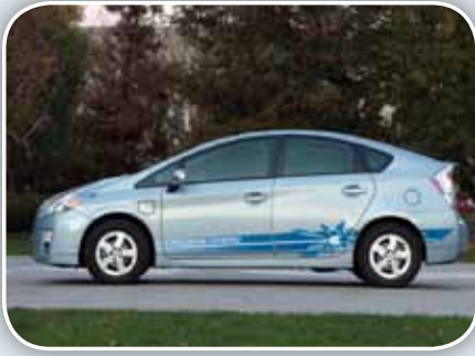
The plug-in hybrid version of the Toyota Prius, the top-selling hybrid in the U.S., is due to be released in 2012. It will use primarily battery power at low speeds and rely on its hybrid system and efficient gasoline engine at higher speeds. It should recharge from a 120-volt outlet in 3 hours. Photo courtesy of Toyota.
