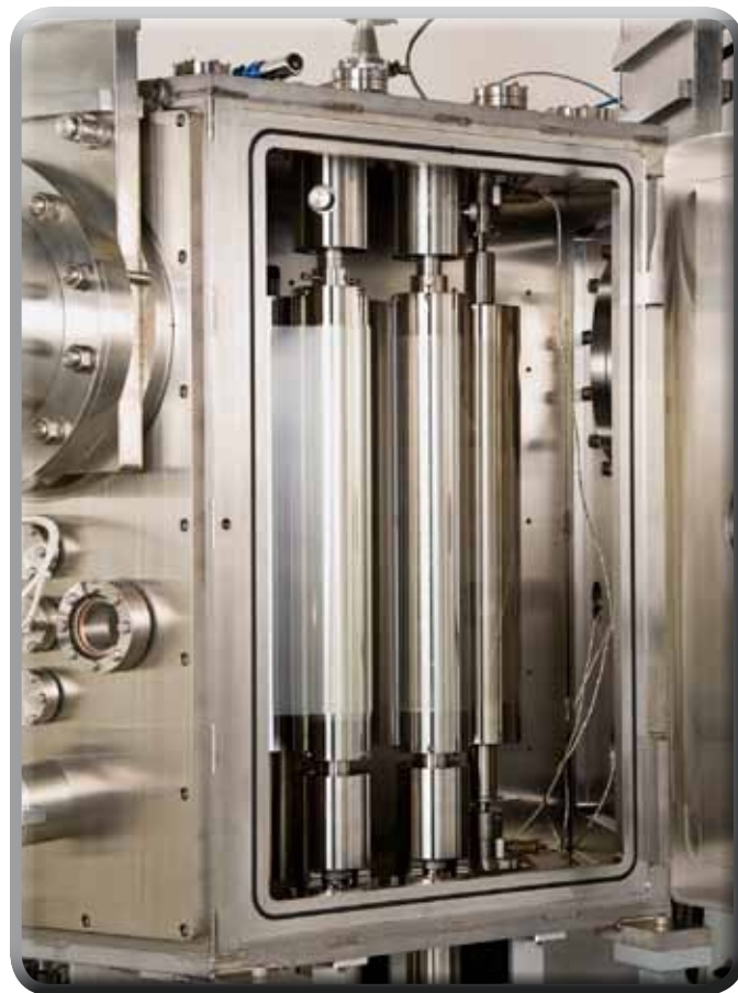
Roll-to-roll production unit for flexible electrochromic coatings
