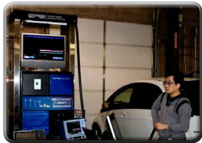
Researchers at EPRI's Knoxville laboratory charge a Mitsubishi i-MiEV with the Utility Direct Fast Charger.
