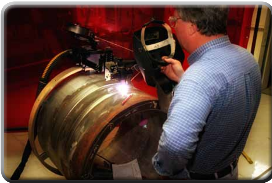
A researcher uses the orbital gas tungsten arc welding process to demonstrate weld overlay application.
