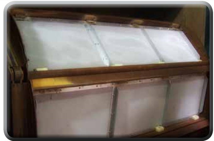
Fine-mesh screen panels overlaid on a coarse-mesh traveling screen assembly
