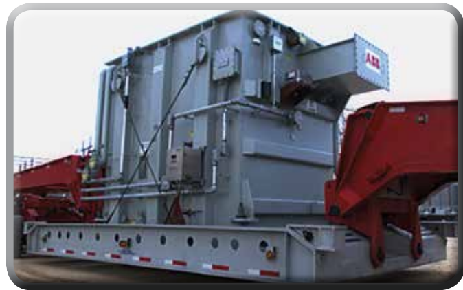
Recovery transformer set up for transport (photo courtesy of the Department of Homeland Security)
