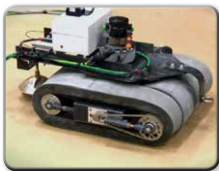
EPRI is developing a lawnmower-sized "concrete crawler" robot to support the safe inspection of large vertical concrete structures in the electric power industry, such as hydroelectric dams, nuclear containment buildings, and cooling towers.
