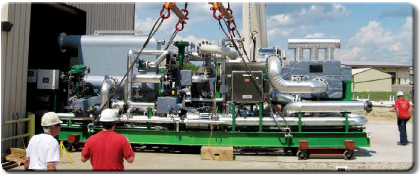
Echogen prototype 10 MW closed Brayton cycle process skid. Used with permission from Echogen Power Systems, LLC (2014)
