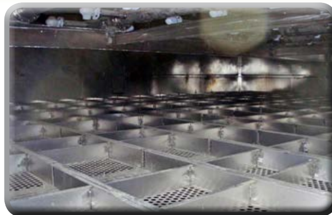
Perforated trays can be used in absorbers to increase contact between flue gas and slurry. Source: Sargent & Lundy
