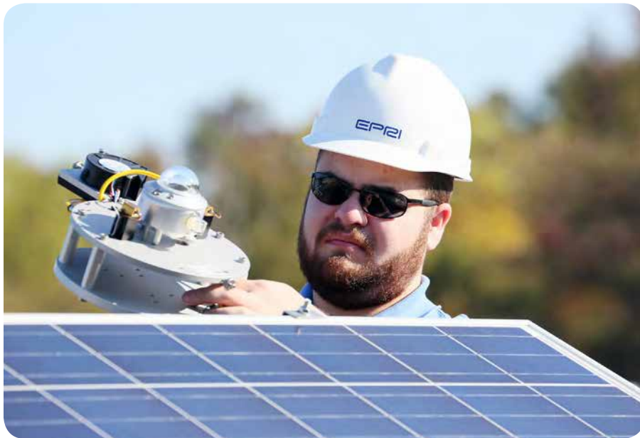
EPRI technician Daniel Foster aligns a pyranometer (an instrument that measures solar irradiance) for one of the 30° fixed-tilt solar arrays.
