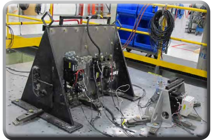
A shaker table test setup for parts called contactors, which are used to start and stop motors
