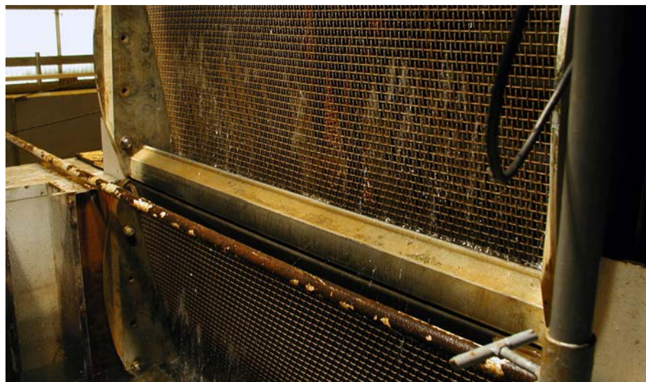
A traveling water screen in a laboratory
